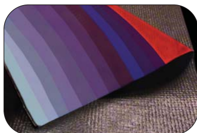
12 Layers of multi-directional TLFP without coated fiberglass reinforcement
