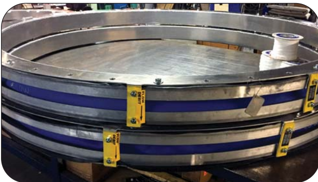
Thorburn's Flexi-Duct™ expansion joints manufactured with Aluminum 6061-T6 (SB-209) frames & backing bars to resist corrosion and reduce weight on the aluminum ducting system
