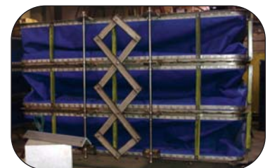
Thorburn's Flexi-Duct™ tertiary expansion joint with a pantograph support system to eliminate hotspot and absorb 600mm (24") lateral and 50mm (2") axial deflection
