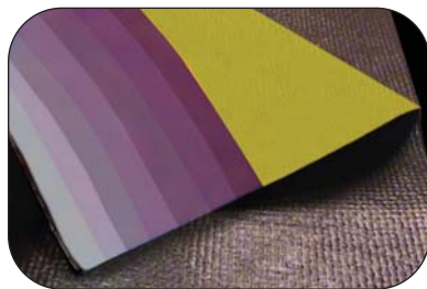
8 Layers of multi-directional TLFP without coated fiberglass reinforcement
