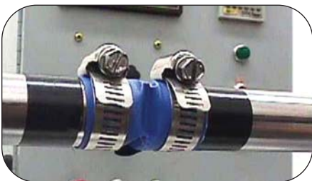
ASTM D2176 Cyclic Flex Testing of Thorburn's TLFP GSM
