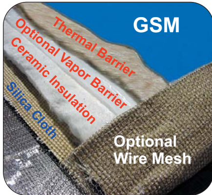
Thorburn's KLFC composite GSM with a stand alone temperature of 1100°C
